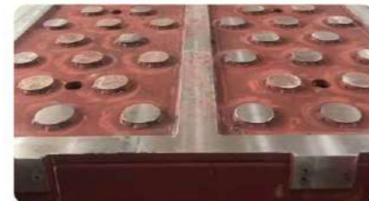
金属真空吸附腔+双层真空吸附 Dual layers vacuum table with metal chamber
