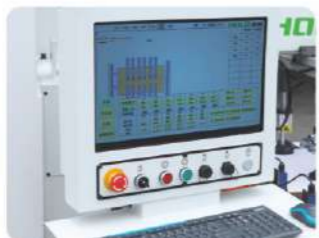
扫码后, 自动显示钻头的分布 After scanning the barcode, the display will show the drill bit distribution
